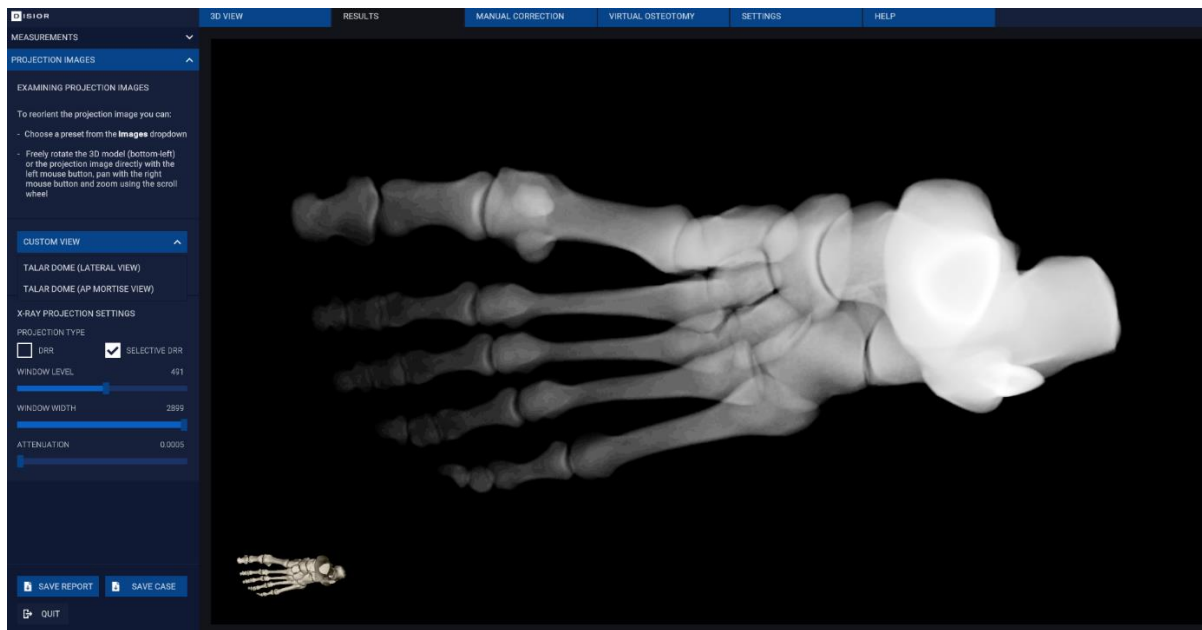
Image 19 Projection images panel on the results sheet for making custom DRRs
